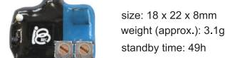
size: 18 x 22 x 8mm weight (approx.): 3.1g standby time: 49h Teleopto receiver 3g / 2ch pulse model: TeleR-3-2P
