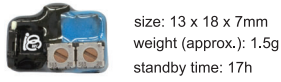
size: 13 x 18 x 7mm weight (approx.): 1.5g standby time: 17h Teleopto receiver 1g / 2ch pulse model: TeleR-1-2P
