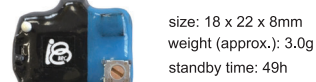
size: 18 x 22 x 8mm weight (approx.): 3.0g standby time: 49h Teleopto receiver 3g / pulse model: TeleR-3-P
