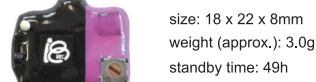
size: 18 x 22 x 8mm weight (approx.): 3.0g standby time: 49h Teleopto receiver 3g / continuous model: TeleR-3-C
